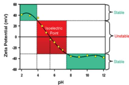
Graph of zeta potential vs. pH showing colloidal stability of aluminum oxide particle in water.
