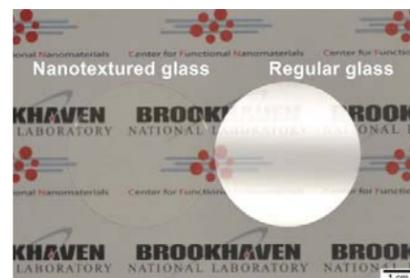
Non-reflective glass will not only benefit consumer electronics, it could be a game changer for solar energy by minimizing the amount of sunlight lost to reflection. It is also a better alternative for pulsed-laser applications, such as those applied to medical devices and aerospace components. As invisible glass is further explored, its use in large scale manufacturing is assured.
