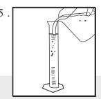
Pour slurry into graduated cylinder to 250 ml mark.
