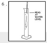
Place hydrometer in slurry and take reading. Adjust as necessary.
